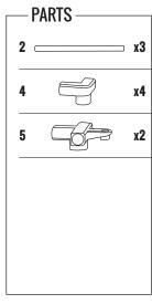
Connect the Table Top Tubes (#2) together by using the Middle Joints (#5) and the Corner Joints (#4).
