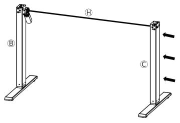
After completing the previous step, insert leg C into the hex stick.
