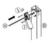
Then, insert the convex end of the motor into leg B together with the motor. Tighten the motor on leg B with the screws shown in the picture.
